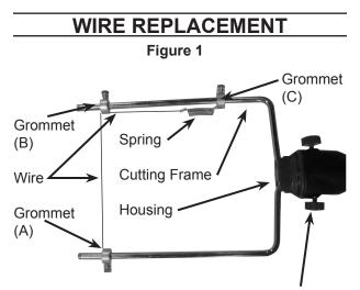
Knobs for holding Cutting Frame to Housing. These are NOT to be adjusted.
